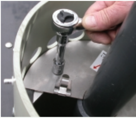
Remove 2 Bolts In Access Plate
